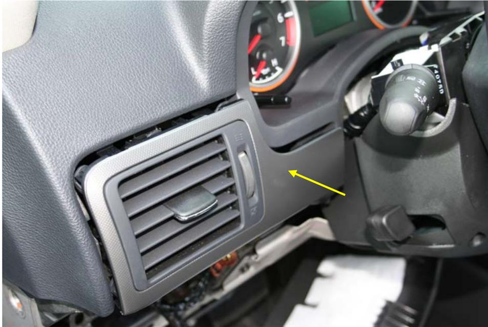
6. Remove the Upper Instrument Panel bezel from the dash:
