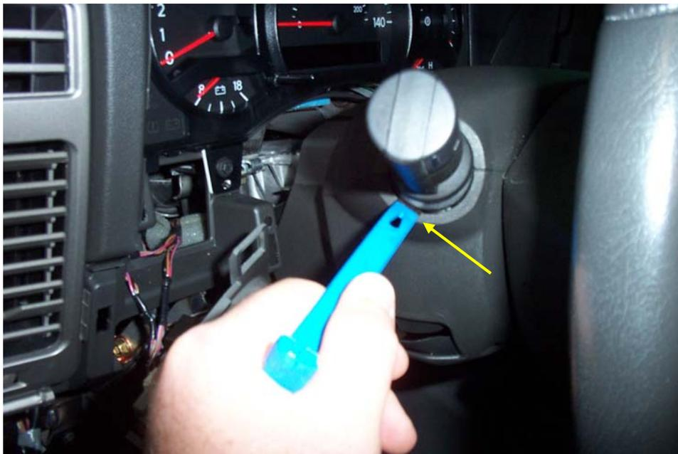
3. Remove the lower Instrument Panel bezel. There are 2 Phillips screws to remove, and then carefully separate the panel from the dash. There are electrical and brake cables connected to this panel, when separated just lower to the floorboard.
