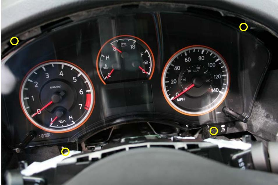
8. Disconnect the factory cable from the Instrument Panel. Press the release mechanism, and gently pull straight out from the instrument panel. To prevent damage, do not rock the connector.
